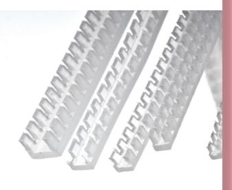
This versatile grommet strip comes in natural coloured polythene, which can be cut easily with a knife or scissors and is fitted without the need for special tools or adhesives. The grommet strip comes in continuous 25 metre lengths, packed in a box for quick, easy and effortless dispensing. It is ideal for circular, oval or irregular shaped openings of all sizes in panels. Available in 9 sizes for panel thicknesses from 0.4 to 12.9mm.
